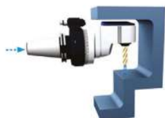
Offset series for machining in narrow spaces with coolant input directly from machine spindle and output through the tool at 70 BAR
