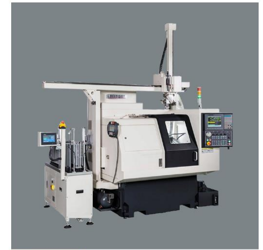
Gantry Loader system
