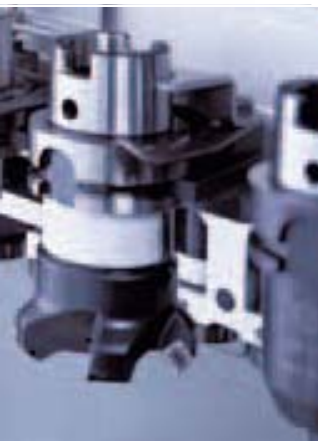
Above: Tool changer chain with 30 pockets and double grippers.
