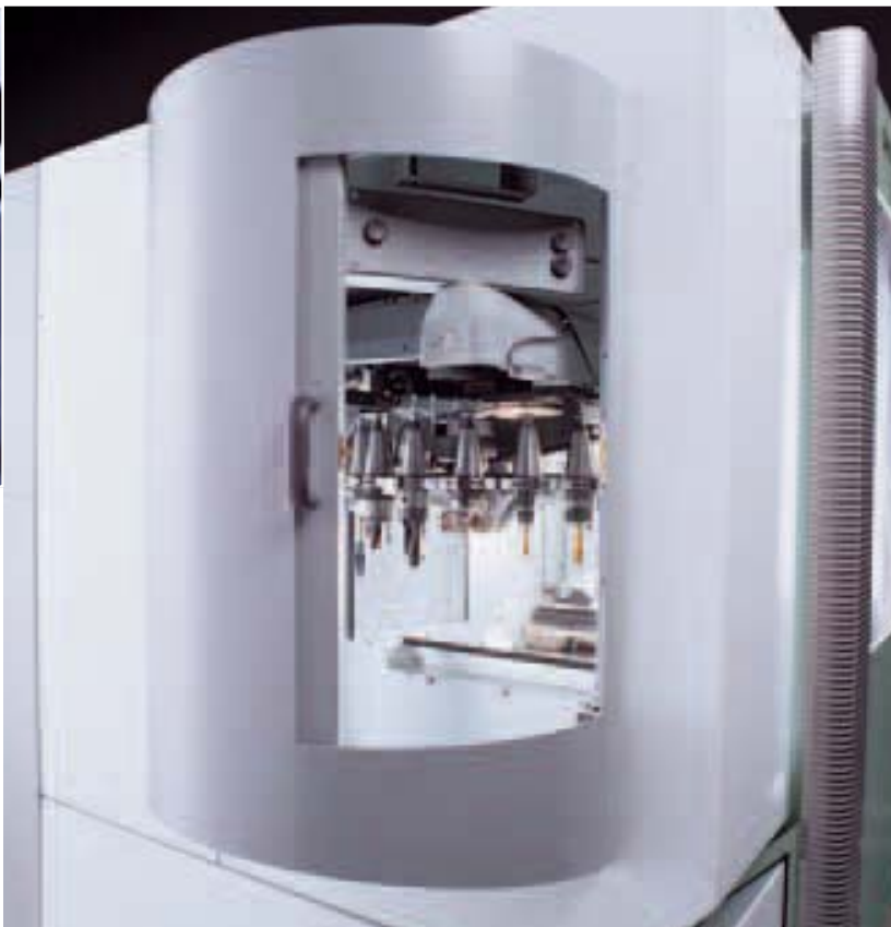
Above: Tool changer chain with 30 pockets and double grippers.
