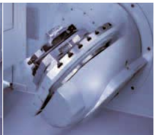
Swivel rotary table with digital drives.
