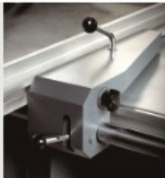
森尺座微调装置 The mintrim device of guide rule
