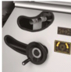
手动升降和角度调节装置 laborate 4000 efficient and angles adjusting equipment
