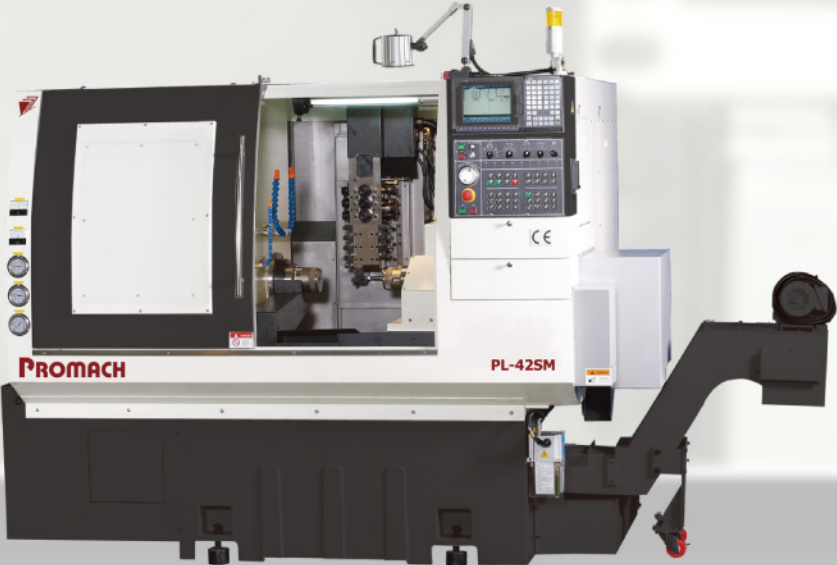
PL series Twin spindle machine equipped with 9 axes to maximize productivity and efficiency
