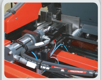
Servo Kontrollü Arka Mengene Servo Controlled Rear Vise
