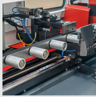
Servo Kontrollü Arka Mengene Servo-Controlled Rear vise
