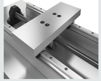
Servo Kontrollü Mengene Hareketi Servo-Controlled Body Movement
