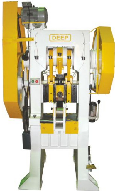
Deep Drawing Double Action Press
