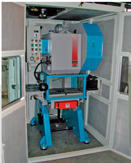
► 27.6T PRESS with soundproofing cabin
