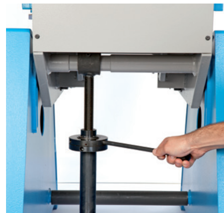
Inclination adjustment (hydraulic on 50 and 88T)
