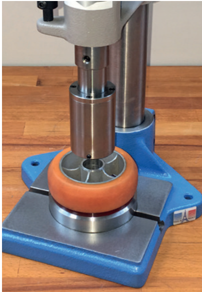
► 4HR with bearing mounting tooling
