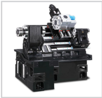
Rigid true slant bed casting, direct coupled ballscrews, with roller style linear guides.
