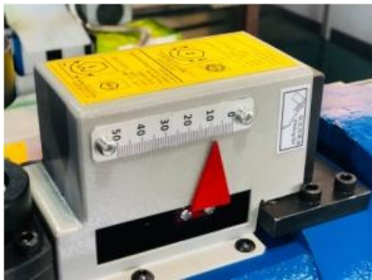
深度调节机构 Depth adjustment mechanism
