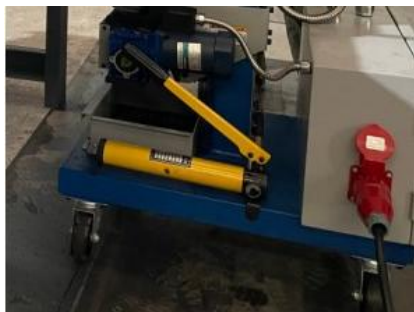
自行机构和升降机构 Self propelled mechanism and lifting mechanism
