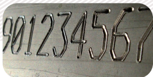
Deep marking on steel
