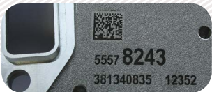
Marking on rough casting
